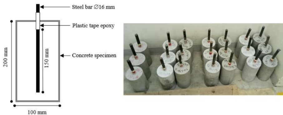
Figure 3. Specimens for corrosion test.
